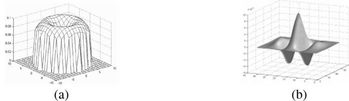
Figure 2: (a) A bandpass filter (from [Wang, 04]), and (b) an even symmetric Gabor filter (from [Jain, 97]).
