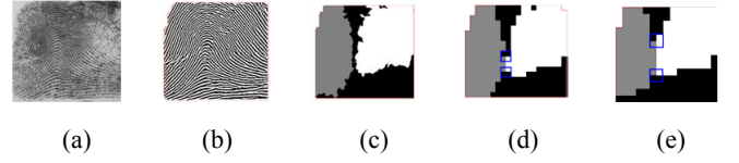
Figure 8 (b) is the binarised image of (a); higher pyramid levels (d) and (e) Identified SPs, but do not have associated SPs at lower level (c)
